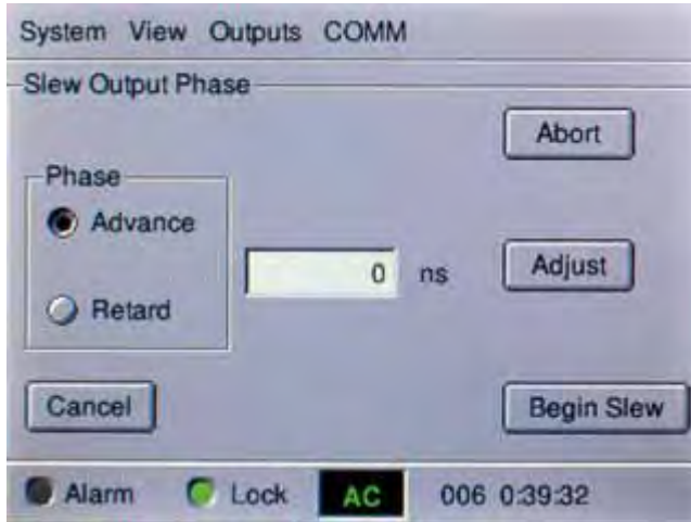
Figure 49 Delta-T (Slew Output Phase)
