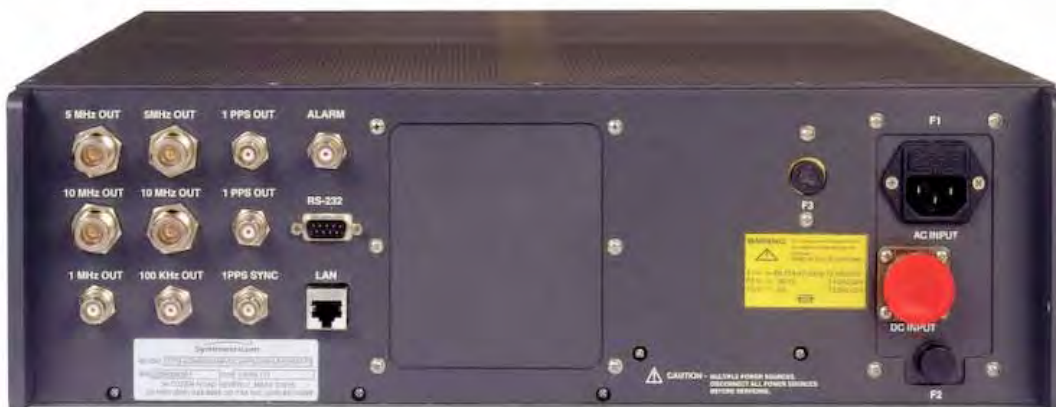
Figure 2 Cs4000 Rear Panel w. Optional Ethernet Port (DCC Option)
